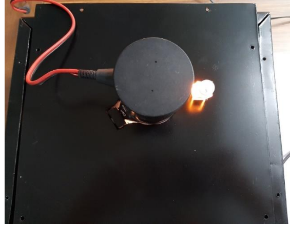
Figure 4.15 Top view of the actual prototype of the NIR spectrometer setup inside the enclosure
