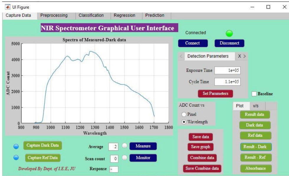
Figure 4.7 GUI developed for the NIR spectrometer using MATLAB App designer. Here the data capture tab is shown.
