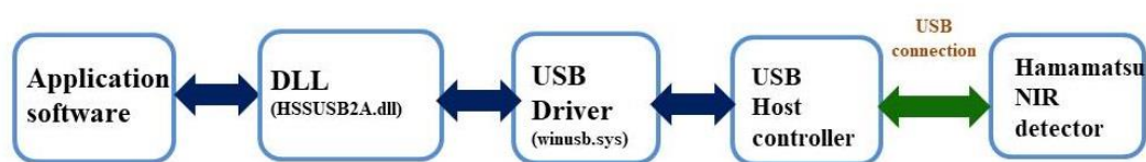
Figure 4. 5 Block diagram illustrating communication between SpecEvaluationUSB2 software and detector.
