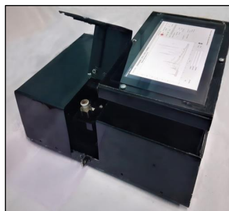
Figure 2. 17 Photograph of the developed prototype portable Raman spectrometer
