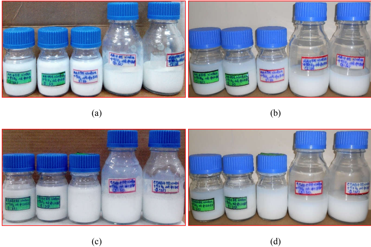
Figure 7 \text{TiO}_2 AA nanofluids (a) freshly prepared, and (b) after 15 days; \text{TiO}_2 CTAB nanofluids (c) freshly prepared, and (d) after 15 days.
