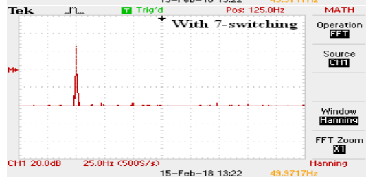
Figure 3. 23 Experimental output for DFIG stator side harmonic spectra before and after proposed switchings (a) at 1520 rpm (b) at 1580 rpm (c) at 1350rpm.
