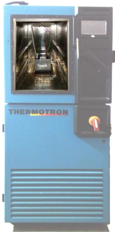
Figure 2.6: Test sample inside the environmental chamber
