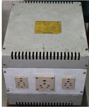
Figure A.5: Isolation Transformer
