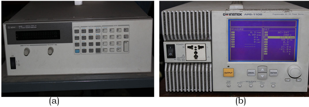
Figure A.8: (a) 6812B AC Power Source/Analyser and (b) APS-1102 Programmable AC/DC Power Source
