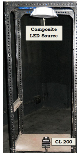
Figure 5.3: Illuminance and CCT measurement setup of test WLED source [Maiti and Roy 2015]
