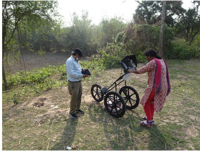
Fig 5.25 GPR survey on Pilkhanar Dhibi, Kankandighi
