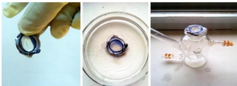
Figure 17: Isolation of Goat's cornea for permeation study across Franz Diffusion cell (Dave et al., 2014)
