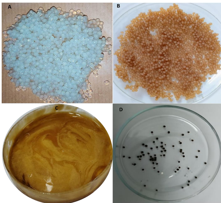
Figure 3: Represents freshly prepared (before drying) (A) Sodium alginate blank beads (B) Sodium alginate loaded with KGS (C) KGS in its traditional form (D) Dried KGS loaded chitosan coated alginate beads.
