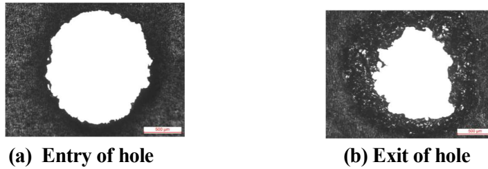
Fig. 5.7 Microscopic views of hole with Straight polarity at 12A/30 \mu s/4s
