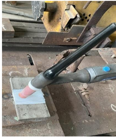
Figure 3.3. Welding torch set above the \text{TiO}_2 flux coated sample before welding
