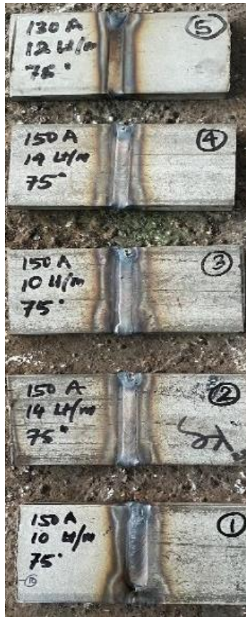
Figure 5.1. Top view of welded specimens of Experiment Set 2
