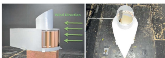
Figure 2.26: Wind turbine with cowling device (Ali et al., 2012)
