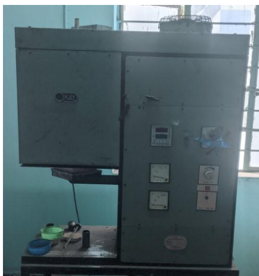
Fig. 4.7: Raising hearth furnace
