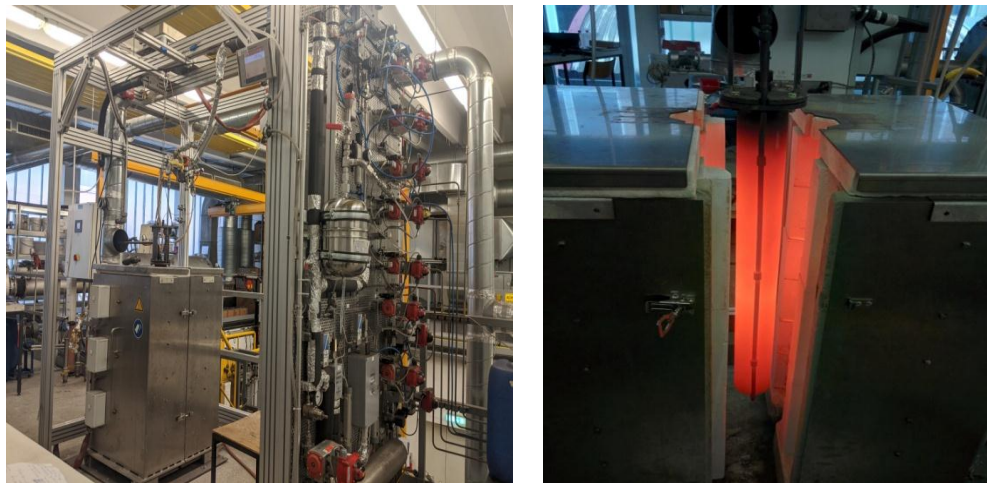
Fig. 4.2: Vertical retort furnace used for tests under blast furnace conditions
