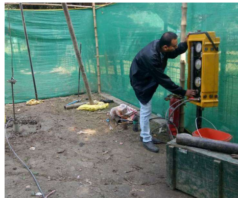
Figure: 3.2 Prebored Menard Pressuremeter (80 Bar capacity)
