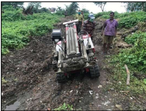
Figure: 3.1 Pagani Penetrometer TG63-150 (150 kN capacity)
