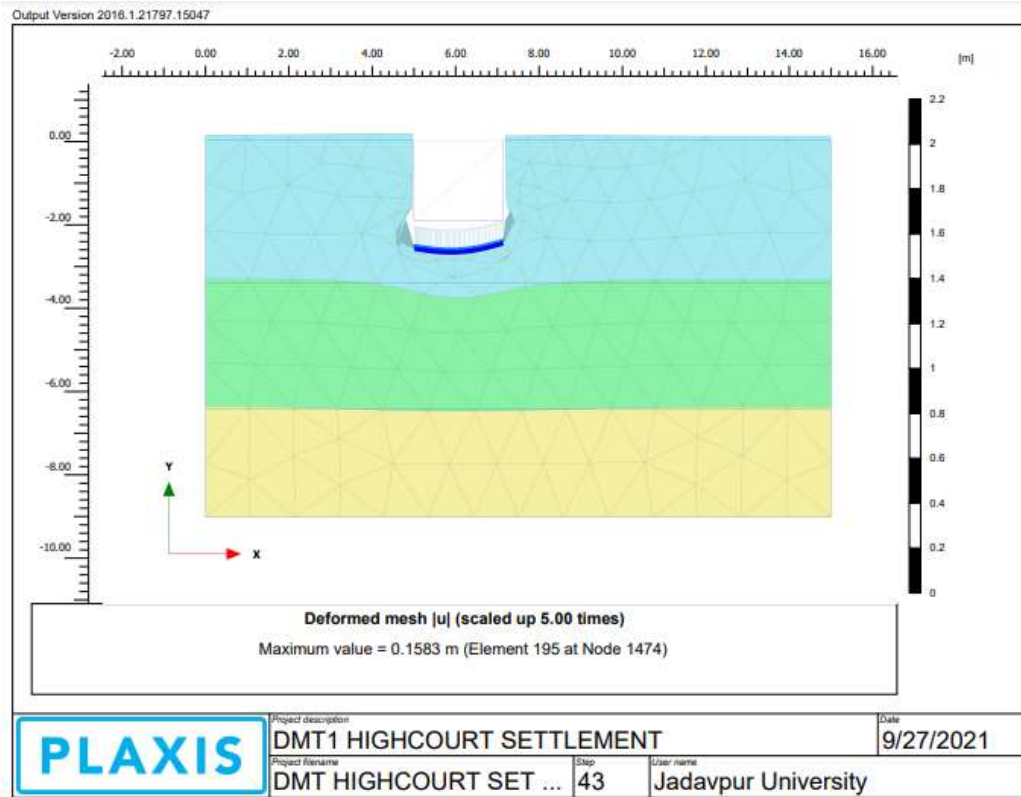
Figure: Appendix-D: 6: Output in Plaxis 2D for modelling based on DMT predicted sub-soil profile
