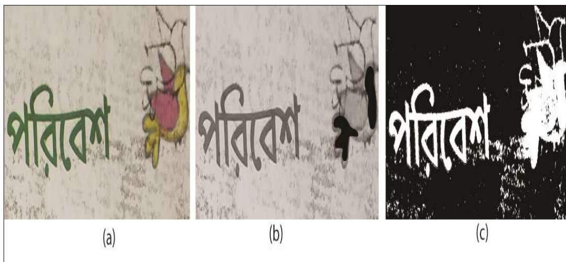
Figure.3.12 Resulted Image of Scumming (Sample 2) (a) Original Image (High Key) (b) Foreground Image (c) Detected Scum Pixels
