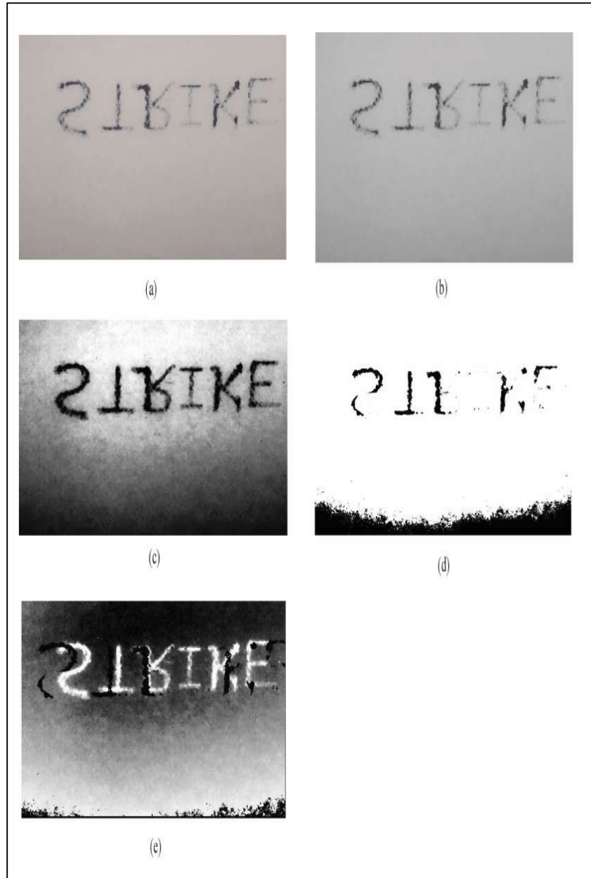
Figure 4.13 Resulted Images of Strikethrough (Sample 4) (a) Original image (b) RGB to Gray Converted image (c) Histogram Equalized Image (d) Foreground Image (e) Detected Strikethrough Pixels.
