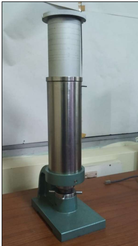
Figure 4.5 Densometer for Measuring the Porosity of Substrate
