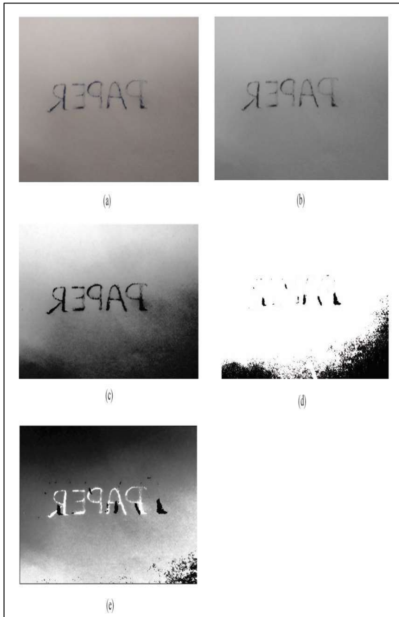
Figure 4.12 Resulted Images of Strikethrough (Sample 3) (a) Original image (b) RGB to Gray Converted image (c) Histogram Equalized Image (d) Foreground Image (e) Detected Strikethrough Pixels.
