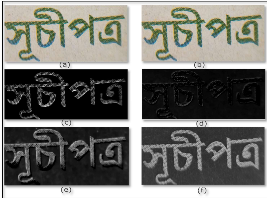
Figure 6.6 Misregistered Sample 3: (a) Original Image; (b) Converted CMYK Image; (c) Image in C-channel; (d) Image in M- channel; (e) Image in Y-channel; (f) Image in K-channel.
