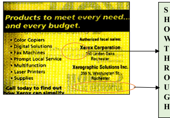
Figure 4.1 Sample Image of Showthrough Printing Defect
