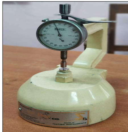
Figure 4.4 Micrometre for Measuring the Thickness of Substrate
