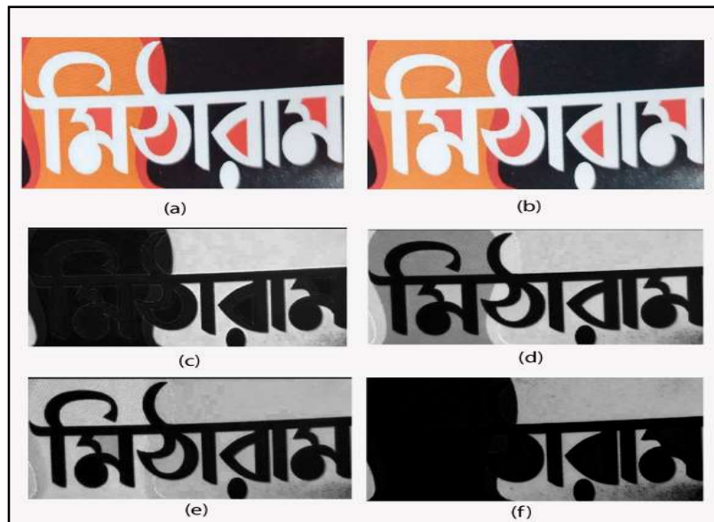
Figure 6.5 Misregistered Sample 2: (a) Original Image; (b) Converted CMYK Image; (c) Image in C-channel; (d) Image in M- channel; (e) Image in Y-channel; (f) Image in K-channel.
