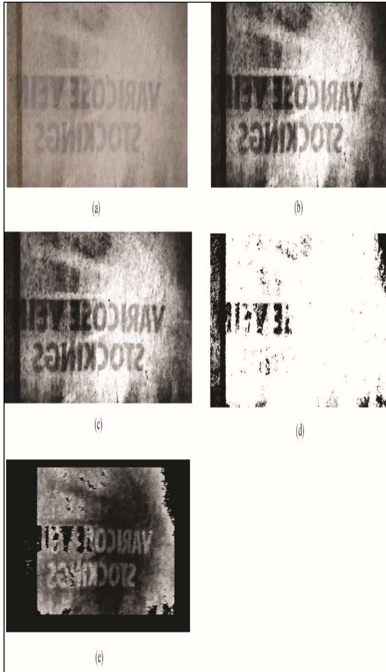
Figure 4.7 Resulted Images of Showthrough (Sample 2) (a) Original image (b) RGB to Gray Converted image (c) Histogram Equalized Image (d) Foreground Image (e) Detected Showthrough Pixels.
