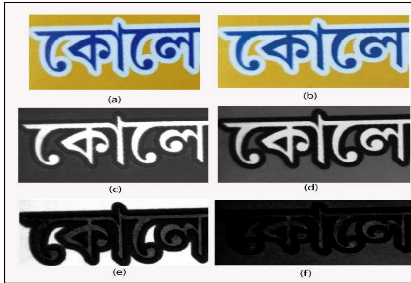
Figure 6.4 Misregistered Sample 1: (a) Original Image; (b) Converted CMYK Image; (c) Image in C-channel; (d) Image in M- channel; (e) Image in Y-channel; (f) Image in K-channel.
