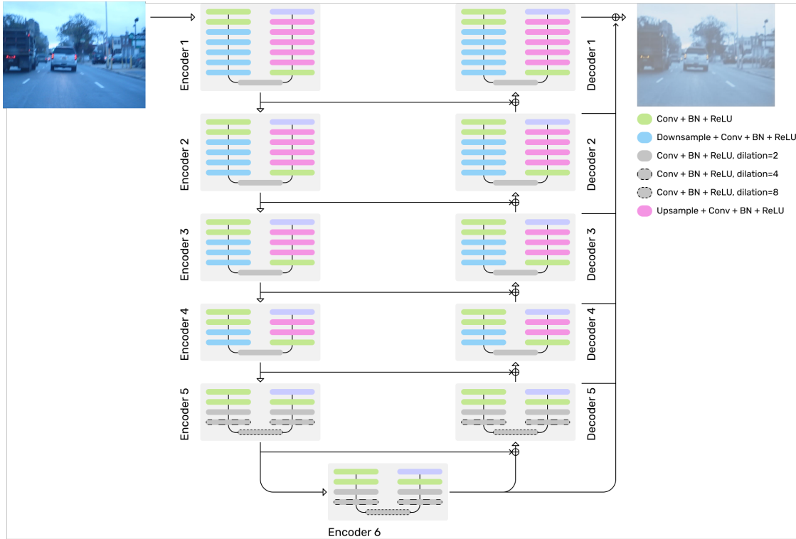
FIGURE 6.1: Architecture of the U^2 model used in the generator of the pix-to-pix GAN model for synthetic hazy frame generation.
