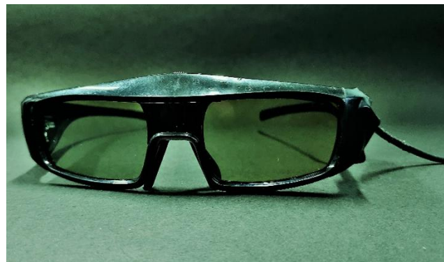
Fig. 5.1 (b): Special Active Shutter Glass
