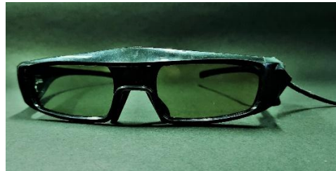
Fig. 4.5 (b): Special active shutter glass
