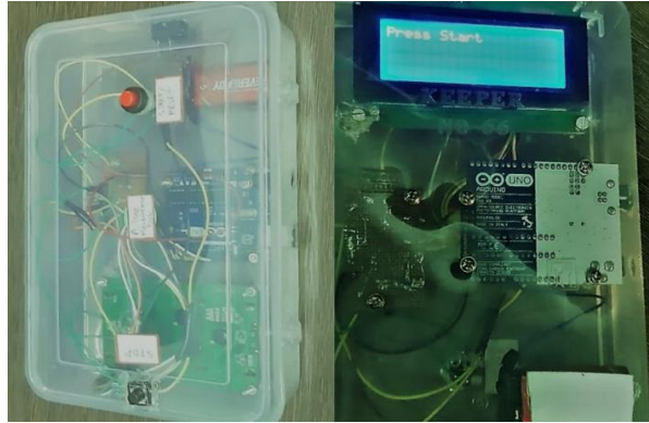
Fig. 4.5 (a): Reaction Time Measuring Compact Device (RTMCD) with Top and Back Side View
