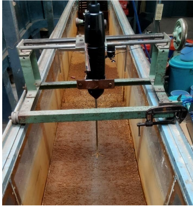
Figure 3.3: Vectrino probe in the flume at Fluvial Mechanics Laboratory, Indian Statistical Institute, Kolkata, India.
