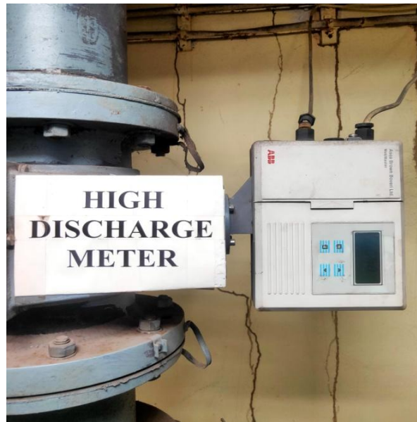
Figure 3.2: Photograph of the electromagnetic discharge meter installed in the Fluvial Mechanics Laboratory, Indian Statistical Institute, Kolkata, India.
