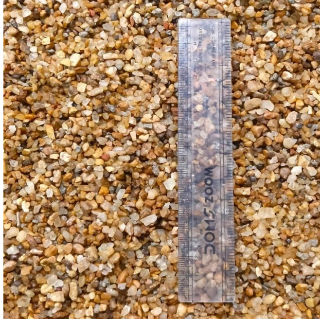
Figure 3.4: (a) Uniform (unimodal) fine sediment with d_{50} = 0.25\text{mm} , (b) Gravel with d_{50} = 3.5\text{mm} in the flume at Fluvial Mechanics Laboratory, Indian Statistical Institute, Kolkata, India.
