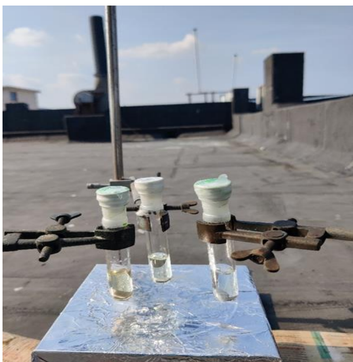
Figure III.41 Photocatalytic reduction of CO 2 in bare sunlight by complex 1a, 2a and 3a .
