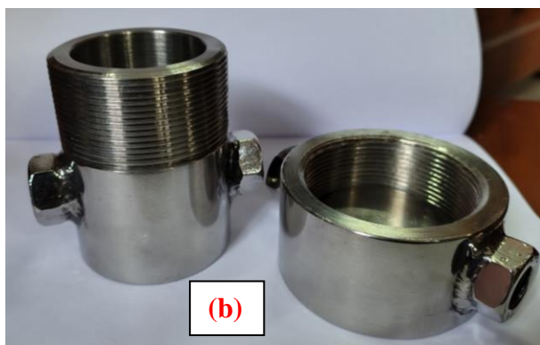
Fig. 15. (a) Hot air ovens used for the solvothermal synthesis technique; (b) The external view of the autoclave used for the synthesis process described in this thesis; (c) The external view of the Teflon vessels used as digestion bombs.
