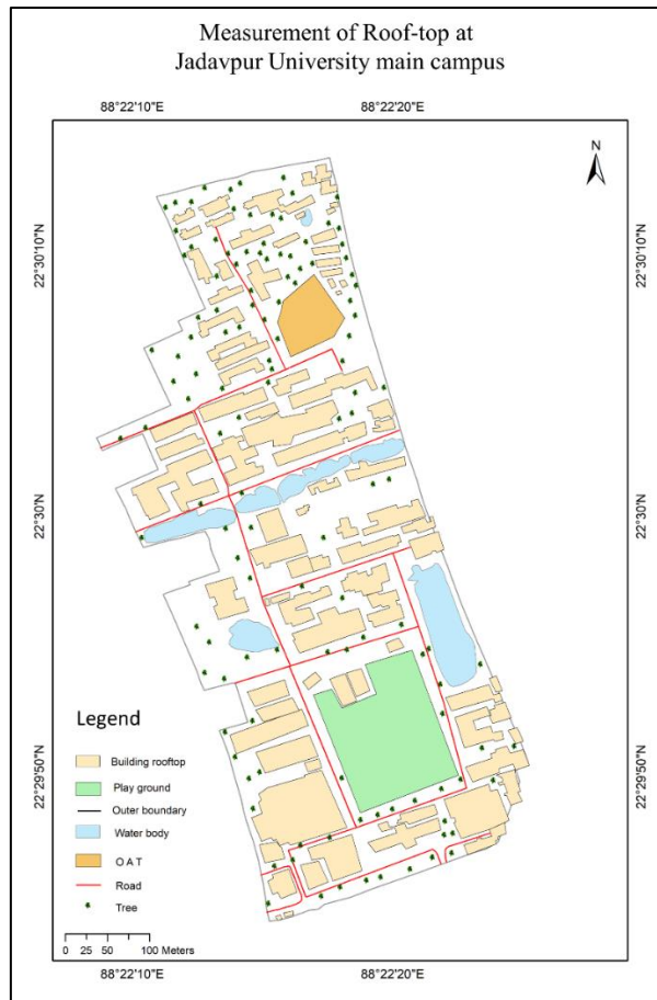
Figure 5.5: Measurement of rooftop area at Jadavpur University main campus, Kolkata
