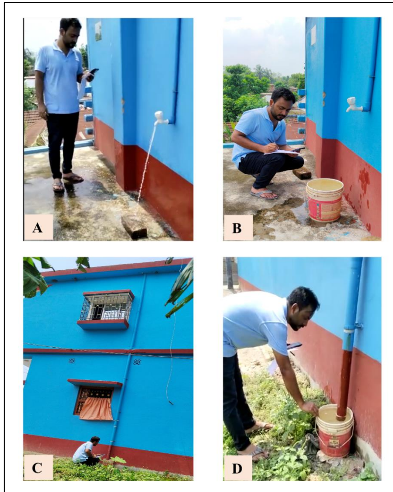
Figure 5.3: Measurement of Runoff Coefficient. A and B illustrate the measurement of water discharge from-a tap, whereas C and D depict the collection of rooftop runoff on the ground.
