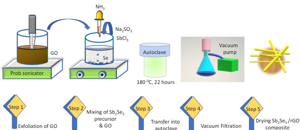
Figure 4.1. Schematic of the synthesis procedure of \text{Sb}_2\text{Se}_3/\text{rGO} hybrid
