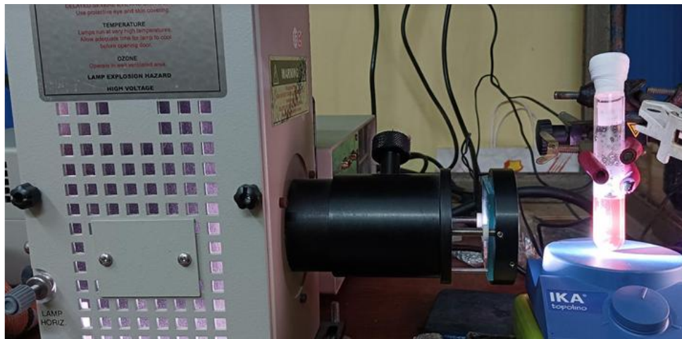
Figure 2.4: Experimental set up of photocatalytic CO 2 reduction reaction.
