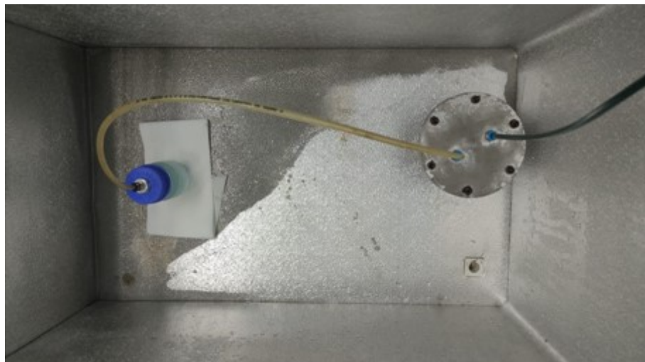
Figure 6.5: The detector and the collecting chamber inside the cold temperature bath.
