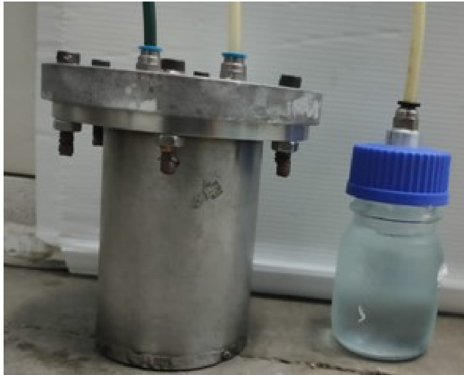
Figure 6.4: The detector and the collecting chamber used in the experiment.
