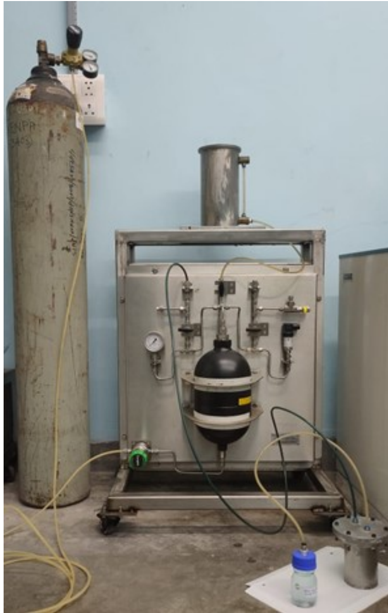
Figure 6.3: The modified pressurization system.
