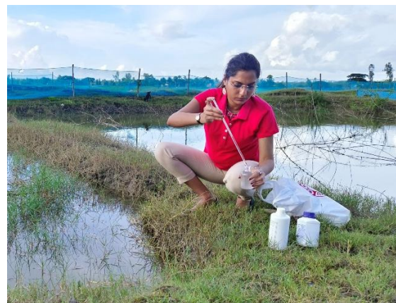
Photograph 5.6: Fixing the water samples in Winkler bottle by adding chemicals for DO analysis.
