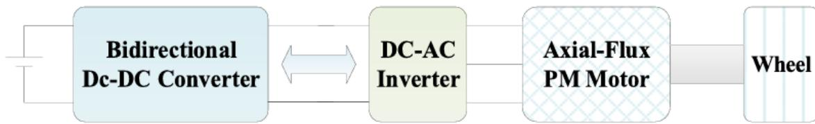
Figure 3.2 Block diagram of a Bidirectional DC-DC converter in EV powertrains
