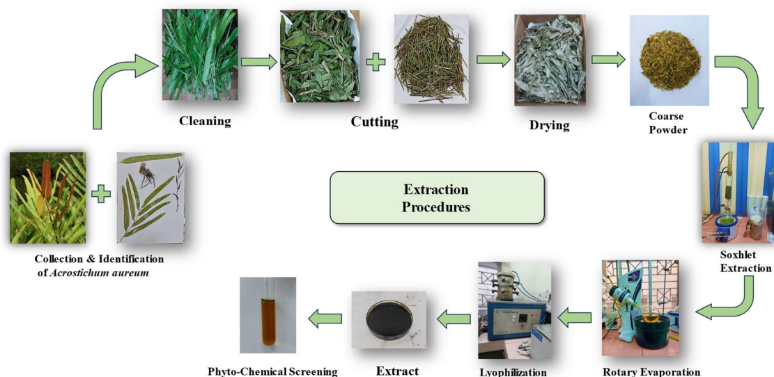
Fig.5: Schematic Diagram of Extraction Procedures
