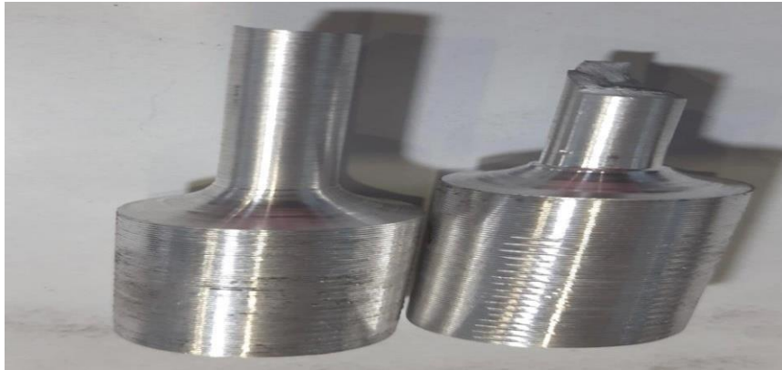
Fig. 24: Fractured test for Sample U after breaking during tensile test
