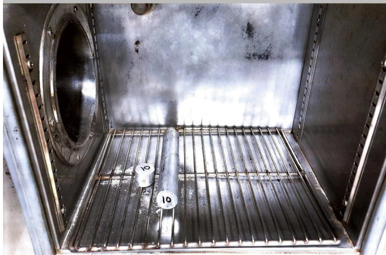
Fig. 10: Tenney chamber used for again heat treatment (-70°C to 200°C)
