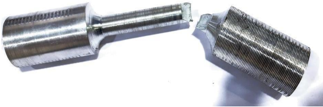
Fig. 26: Fractured test Sample W after breaking during tensile test
