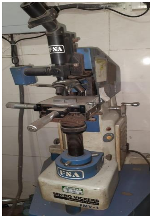
Fig. 29: Micro Vickers Hardness Machine with the sample for measurement of Hardness
