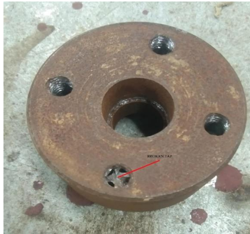
Figure 5.2 JOB WITH INSERTED BROKEN TAP
