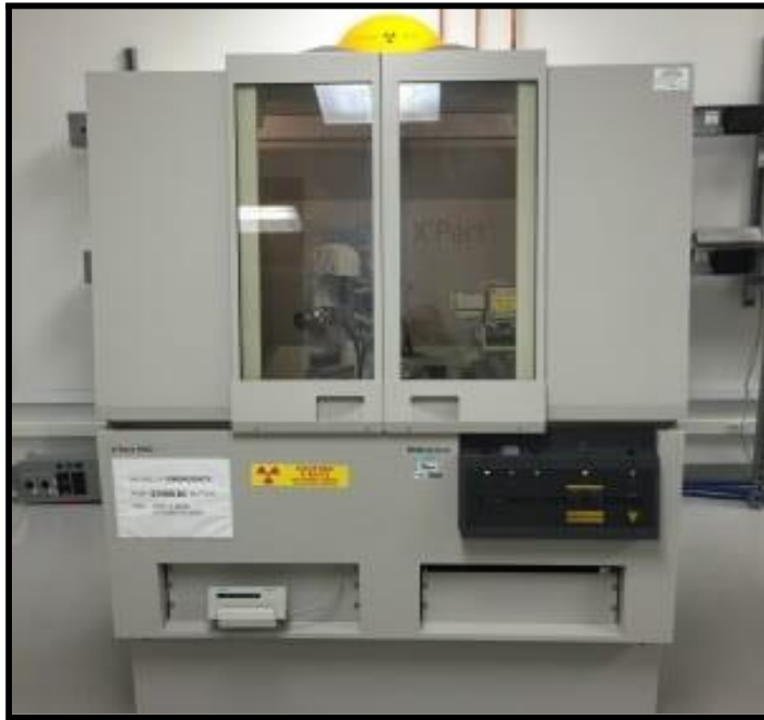
Fig.5 : Picture of XRD machine used for the XRD analysis
