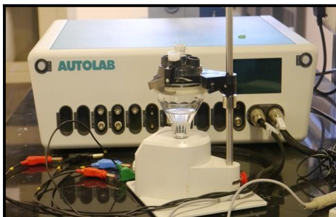
Fig. 8: AUTOLAB corrosion testing machine
