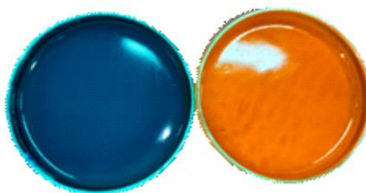
Fig 3.3 Cross-linked hydrogel films dyed with methylene blue and methyl orange indicators for visual inspection of self-healing ability.
