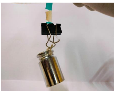
Fig.3.4 Determination of healing efficiency of borax cross-linked hydrogel film through tensile stress
