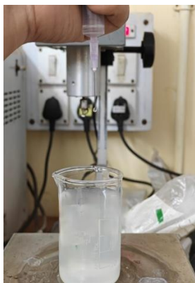
Slowly adding Drug Loaded Sod.TPP solution to Chitosan Solution with syringe
