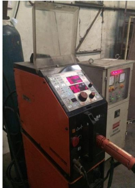
Figure 3.2 For pro mig 530 kemppi MIG welding were used.
