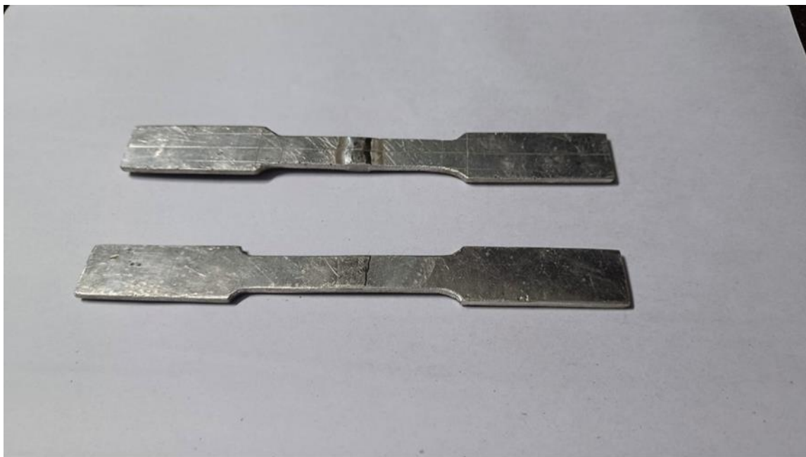
3.8 Figure a) Tensile specimen before test
