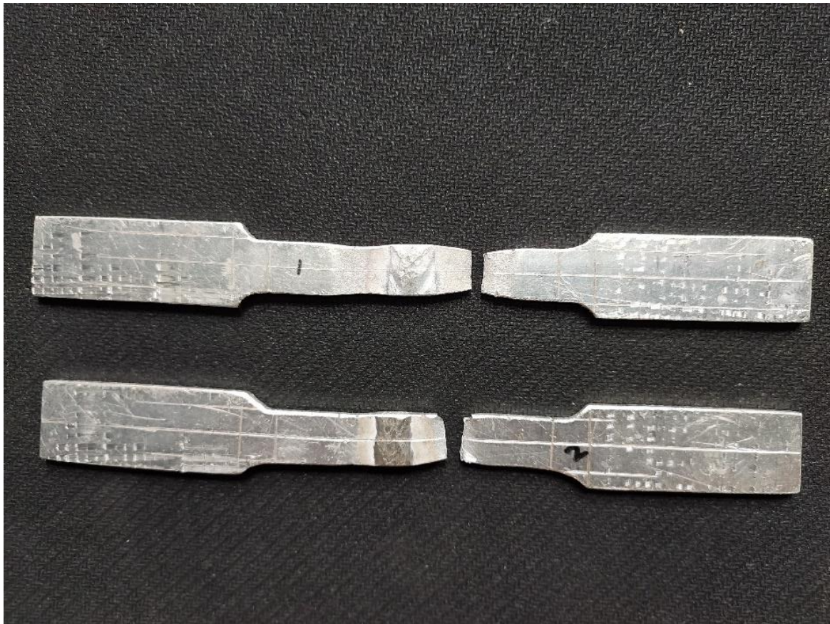
3.8 Figure b) Tensile specimen after test
