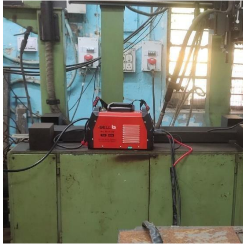
Figure 3.1 For TIG and MMAW welding ibell t250-106
