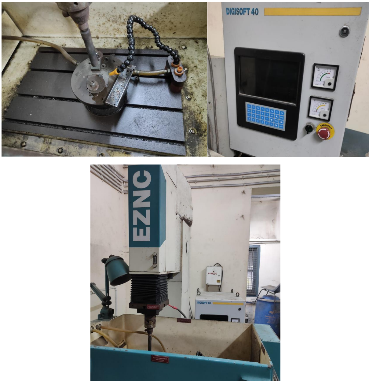
Fig 3.1 Experimental Setup of EDM machine system
