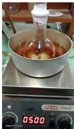
Figure 16: Reaction setup of 5-(4-isopropylbenzylidene) thiazolidine-2,4-dione.
