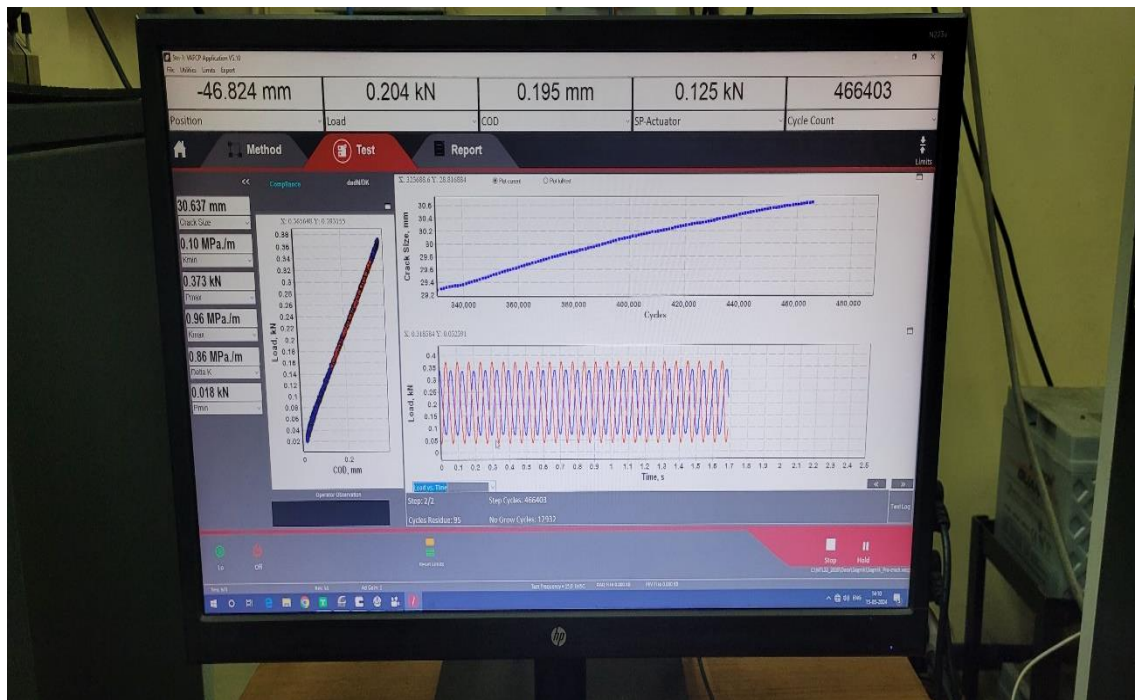
Fig 4.6: Sinusoidal loading applied during testing
