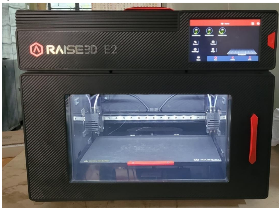
Fig 3.3: FDM printer used for producing test specimens
