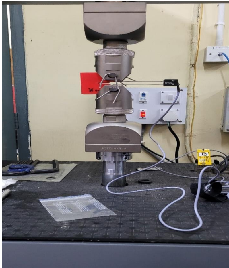
Fig 4.5: FCGR test in progress
