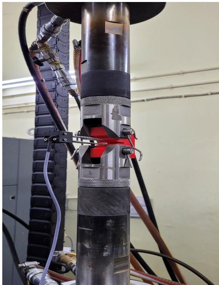
Fig 5.2: Fracture Toughness testing in progress
