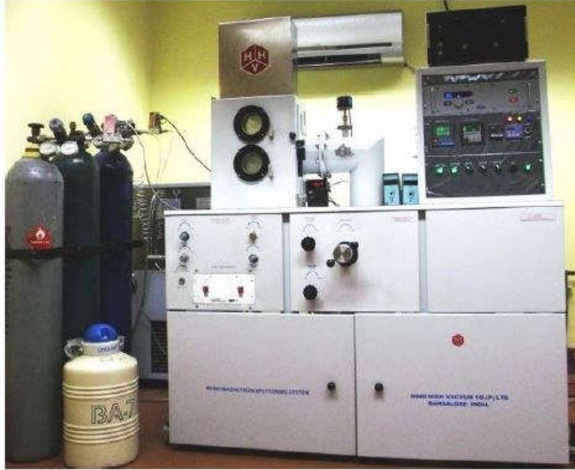
Fig 2.4: Magnetron sputtering system in our lab, used for depositing TCO layers.
