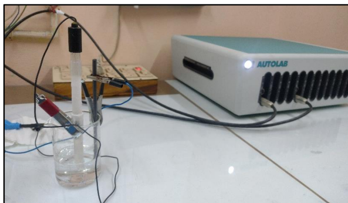
Figure 13: Corrosion Testing Autolab instrument
