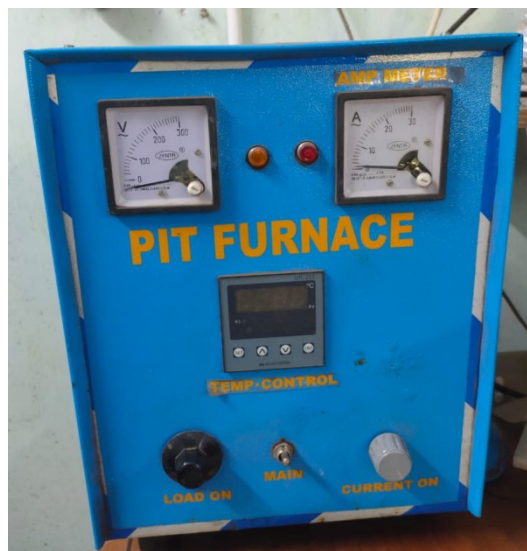
Fig 4.7 : Electrical Pit furnace Table 4.2 : Specification of Electrical Pit furnace
