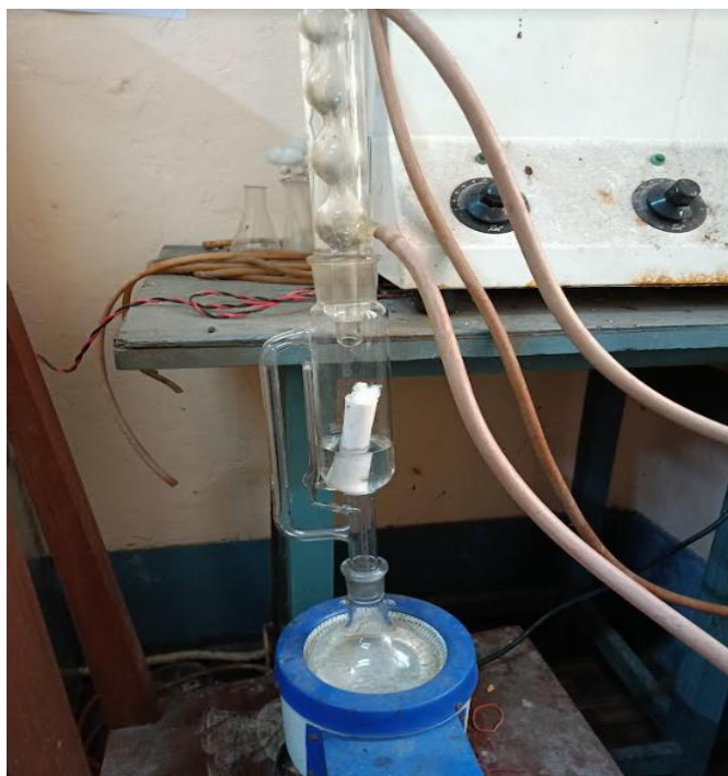
Fig 19: Soxlet Extraction process
