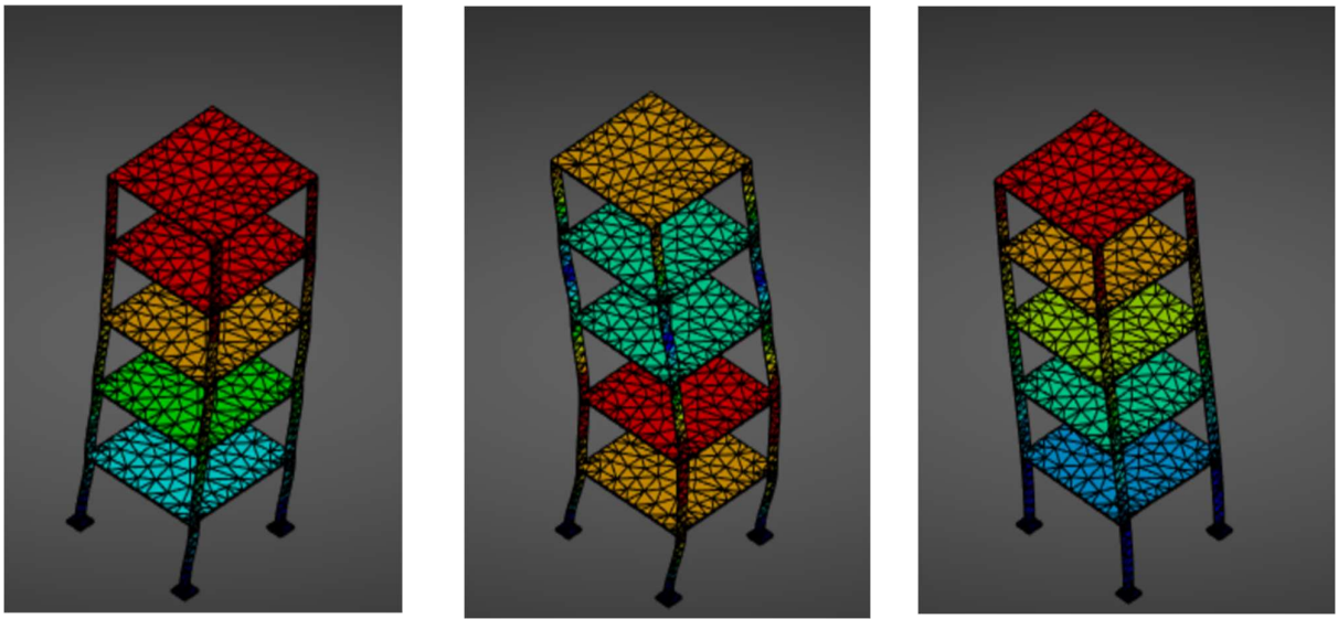
Figure 5.2.- Mode shapes of three different modes
