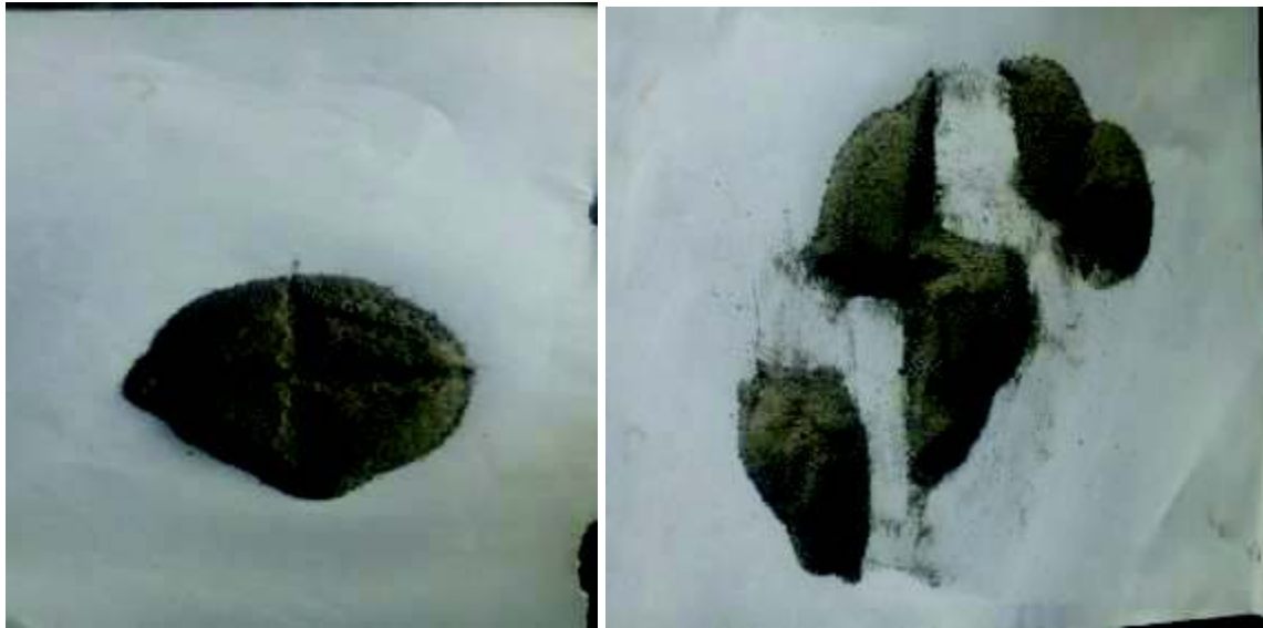
Fig.3.8 Cone and Quartering Method for SEM Sample Preparation
