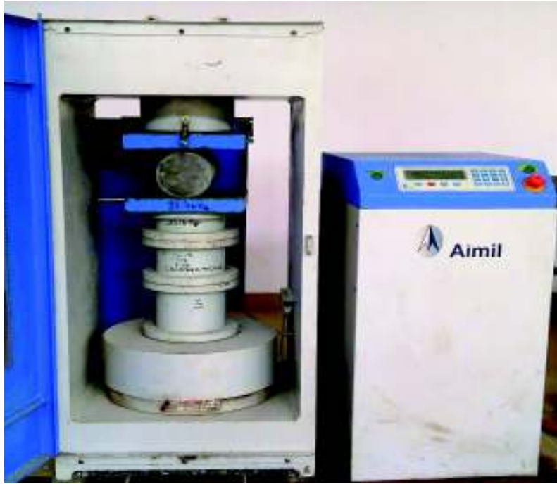
Fig. 3.3 : Split Tensile Strength Test of Concrete
