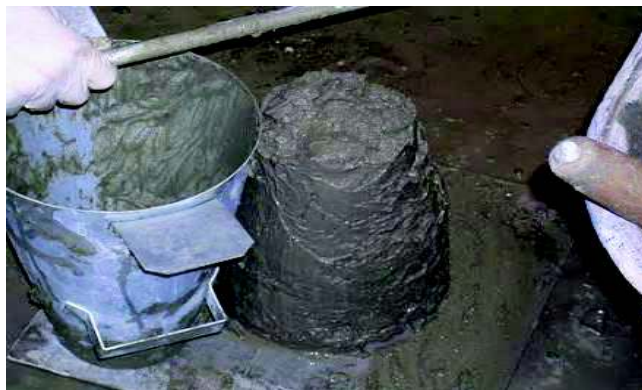
Fig 3.1 : Slump Test of Concrete
