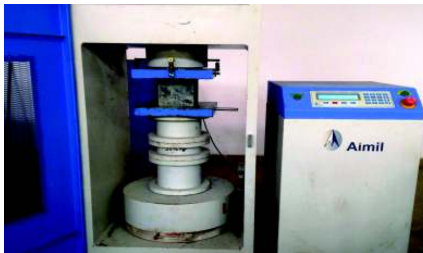
Fig 3.2 : Compressive Strength Test on Compression Testing Machine
