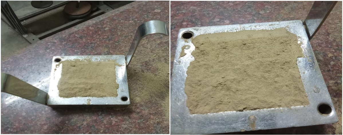
Fig. 3.3.1: Sheared plane view as captured during the test.
