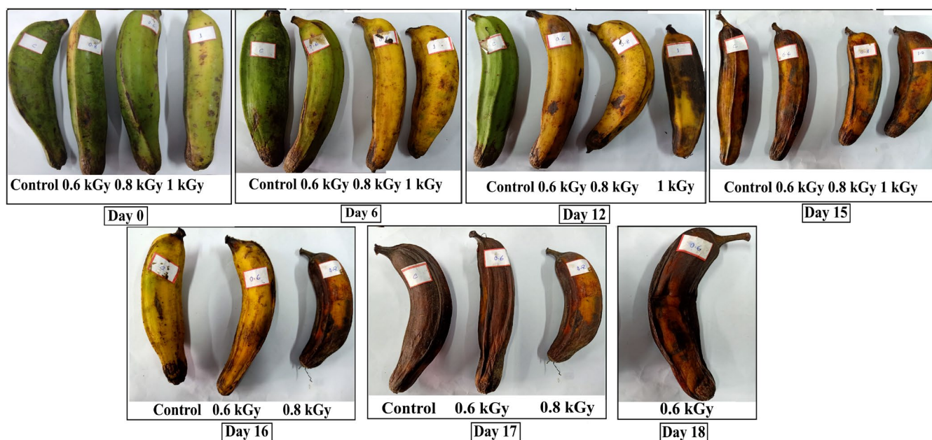
FIGURE 9 Physical changes in \gamma -irradiated (0.6–1 kGy) plantains and control samples during 18 days of storage when stored at 23 \pm 2^\circ\text{C} , 70 \pm 2\% RH in an environmental chamber
