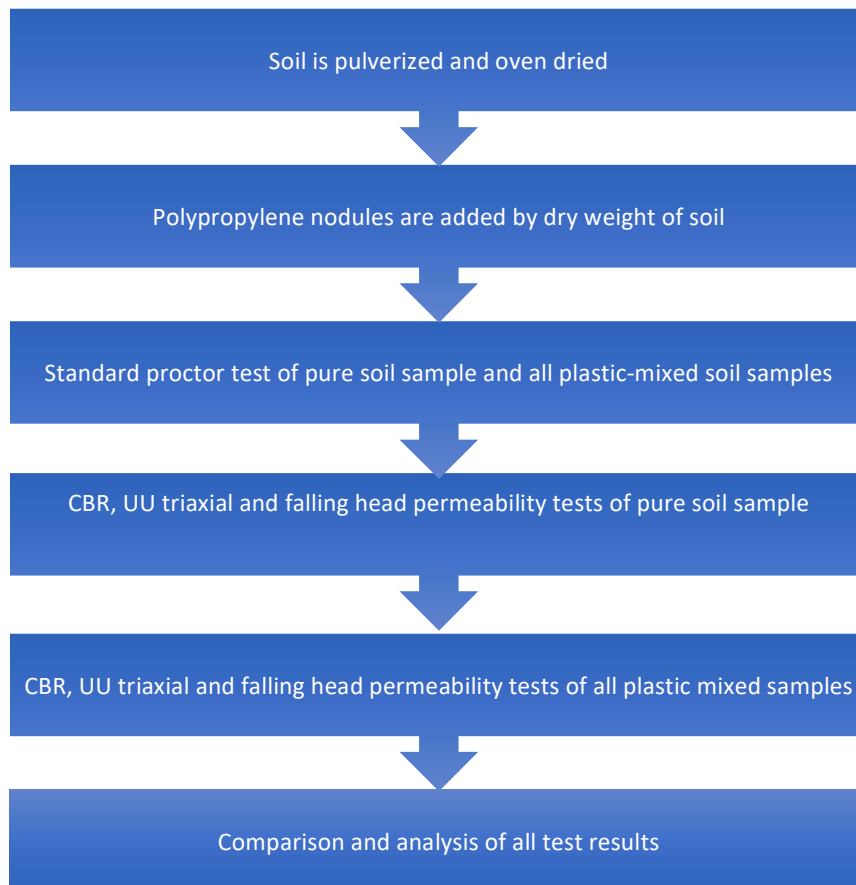
Figure 1- Work plan and flow chart
