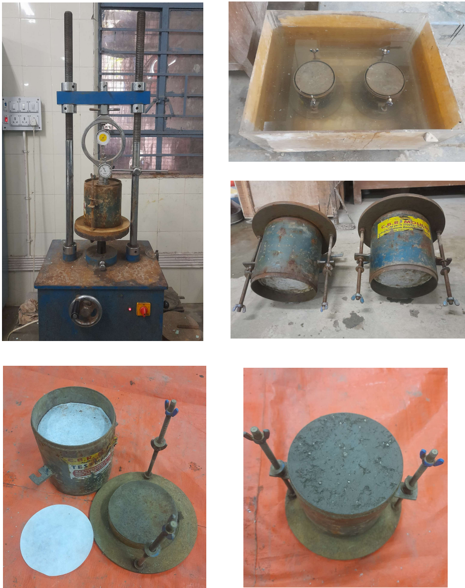
Figure 8- CBR Apparatus and Sample
