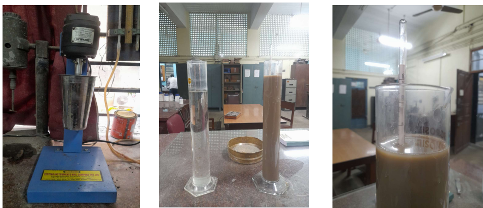
Figure 6- Hydrometer test apparatus and sample
