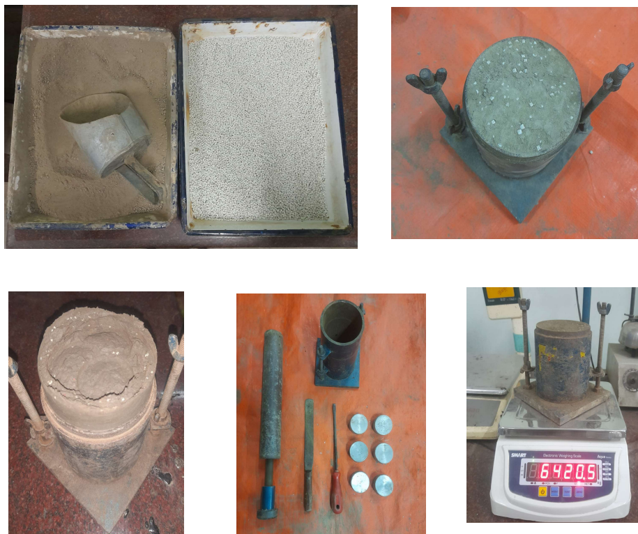
Figure 7- Standard Proctor Apparatus and Sample
