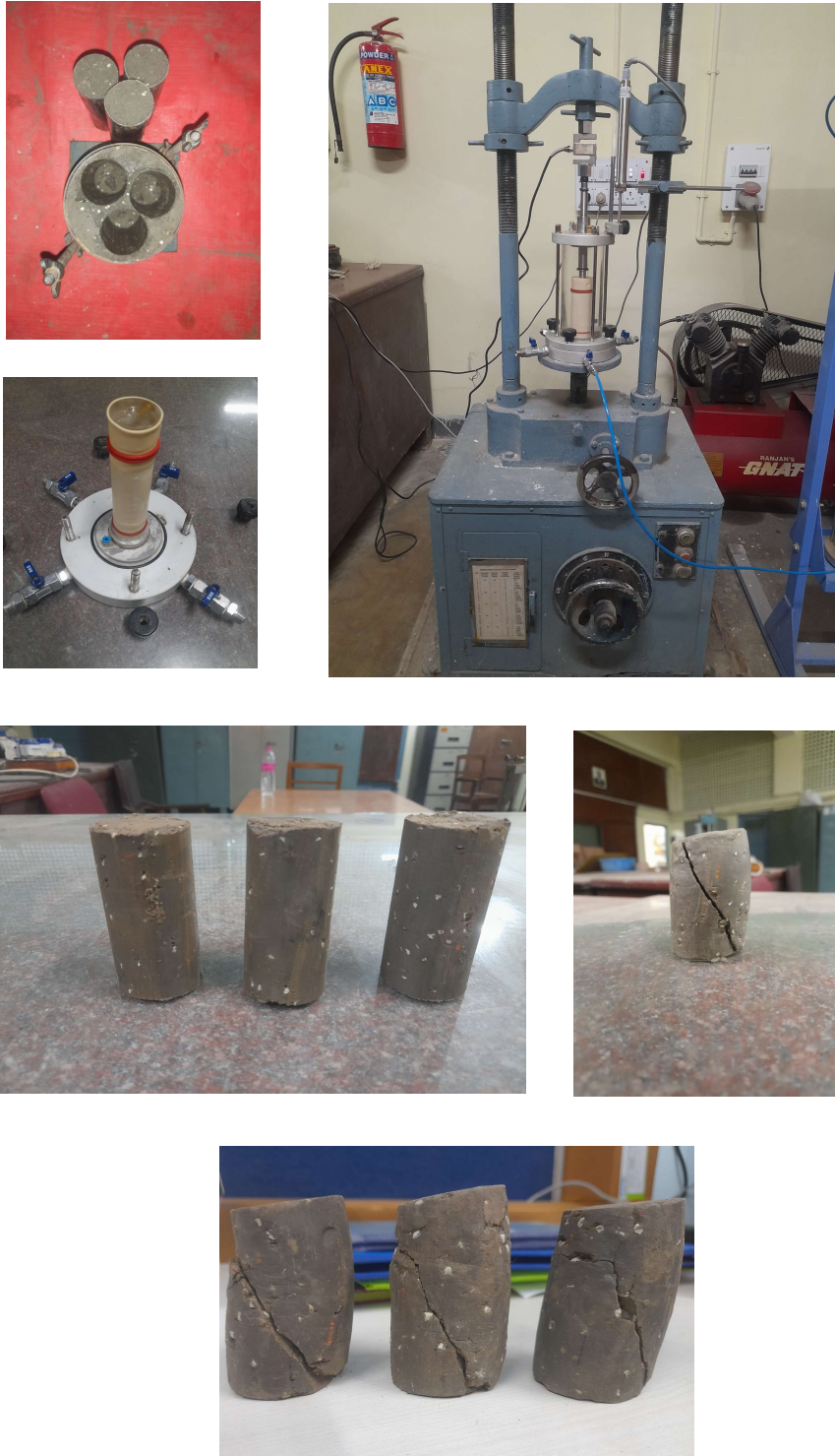
Figure 9- UU Triaxial Apparatus and Sample
