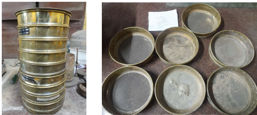
Figure 5- Wet sieve analysis apparatus and sample
