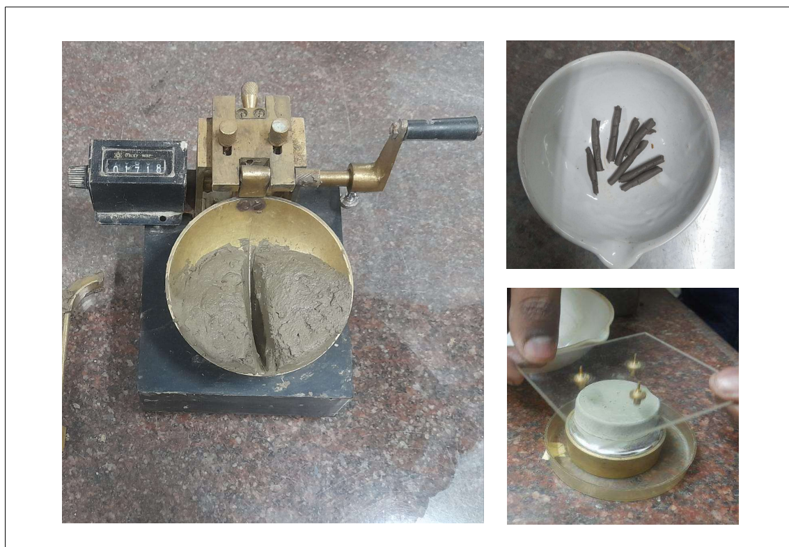
Figure 2- Atterberg limit test apparatus and sample
