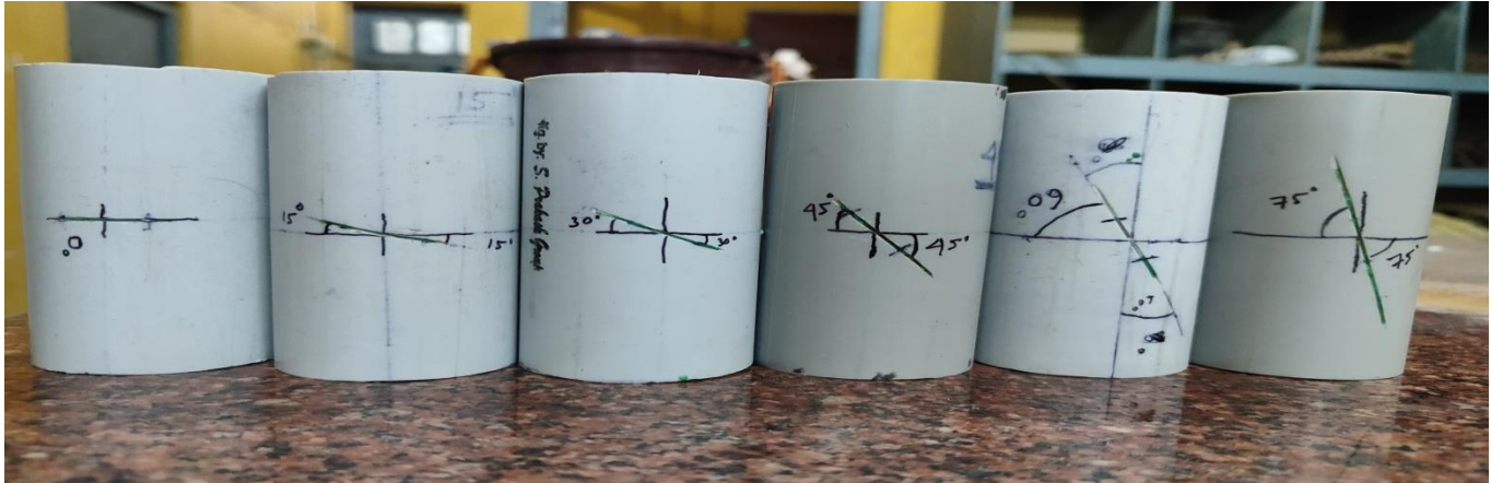
Fig 3.1: PVC moulds with cracks having orientation such as 0^\circ , 15^\circ , 30^\circ , 45^\circ , 60^\circ , 75^\circ for the preparation of rock sample.
