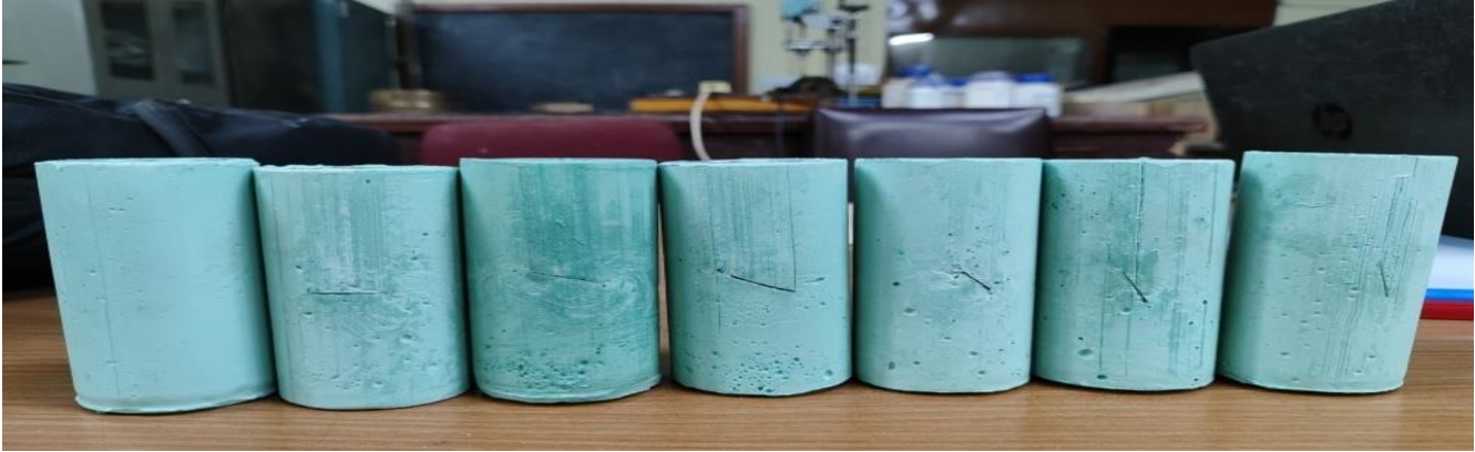
Fig 3.2: Intact rock sample and samples with cracks having orientation such as 0^\circ , 15^\circ , 30^\circ , 45^\circ , 60^\circ , 75^\circ
