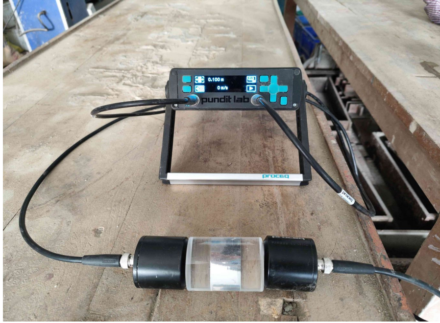
Fig 2: A typical UPV apparatus with calibration rod
