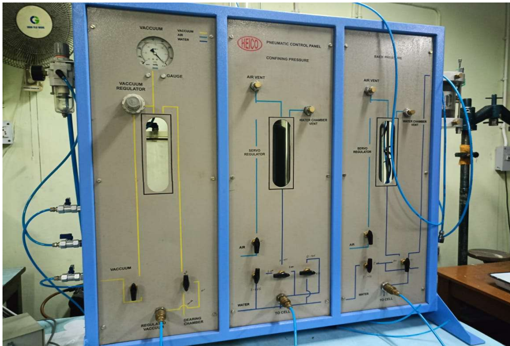
Fig.53: Pneumatic control panel for the application of confining pressure, back pressure and vacuum.
