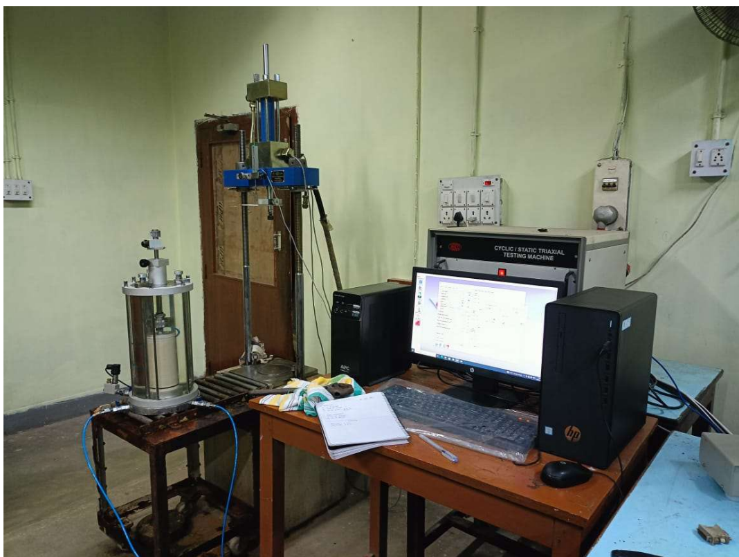
Fig.54: Monitor, CPU, Triaxial Cell and Loading frame
