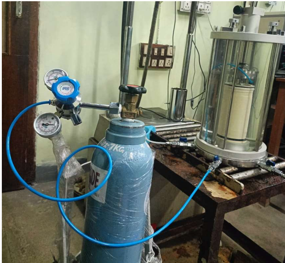
Fig.49 : Process of Saturation of sample by flushing of gaseous \text{CO}_2 through the soil sample
