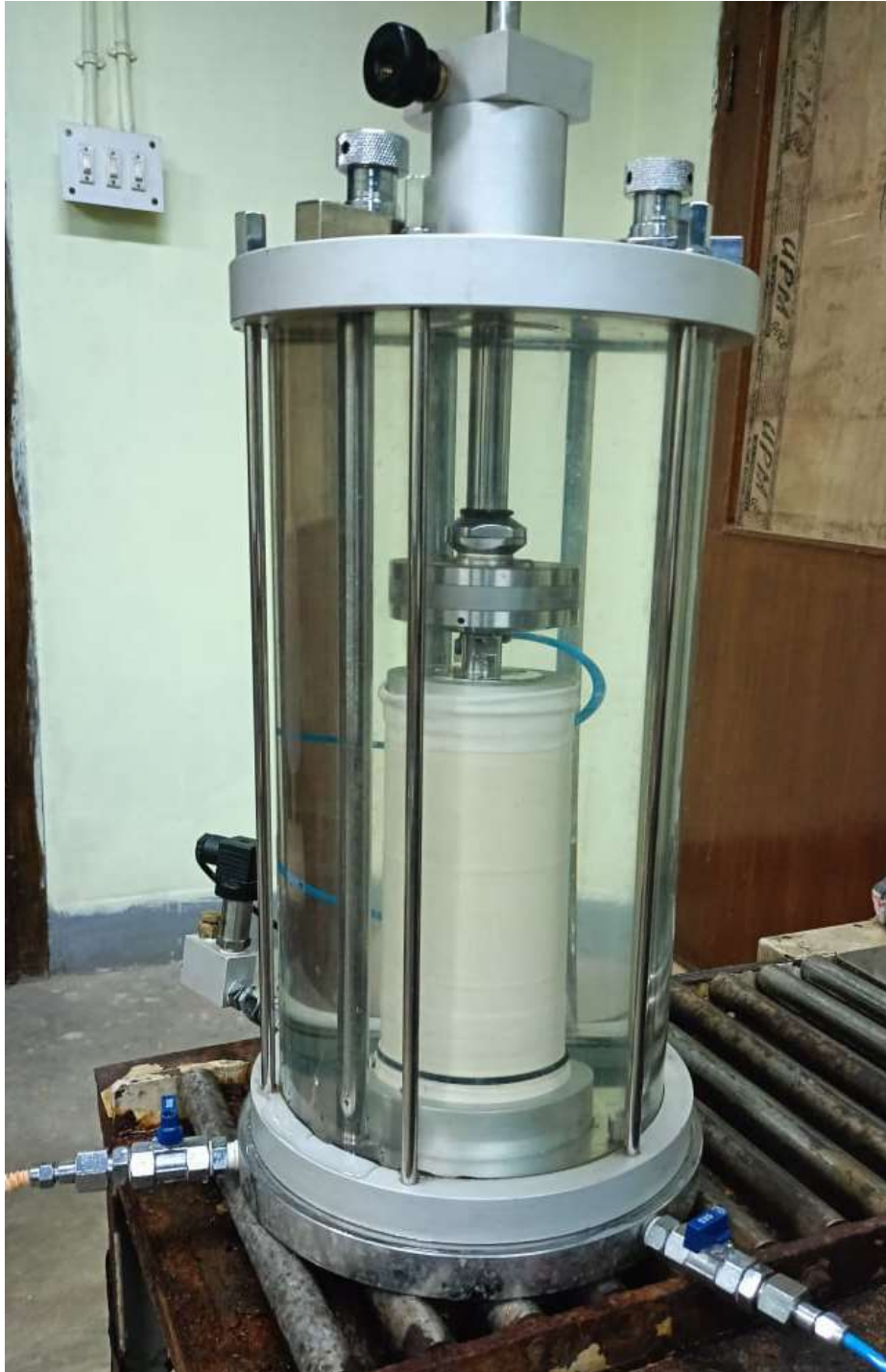
Fig.51 : After completion of consolidation Phase before shearing of the sample
