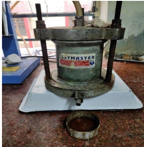
Figure 29: Falling Head Permeameter test apparatus (Jadavpur University, 2024)
