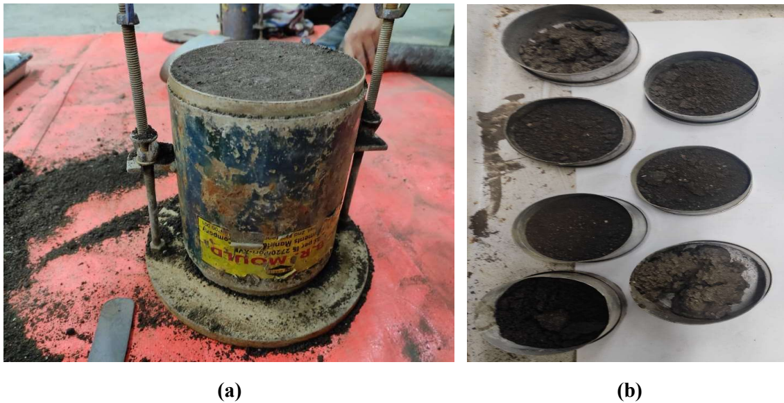
Figure 28: (a)- Proctor mould with compacted sample, (b)- Sample for oven drying (Jadavpur University, 2024)
