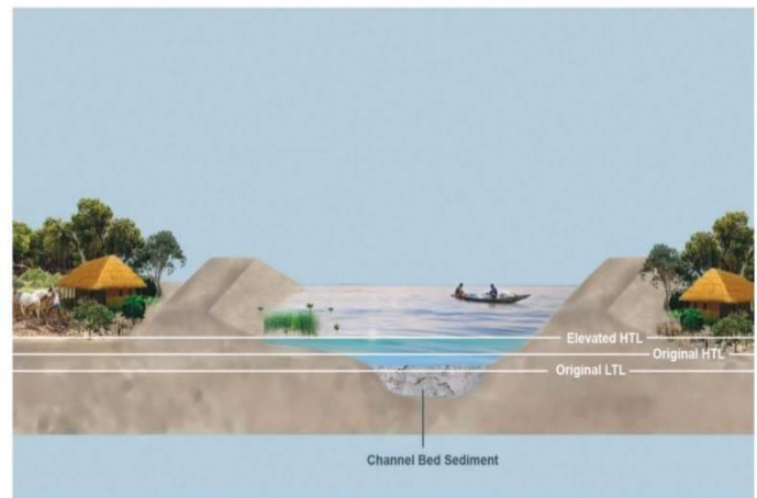
The sedimentation on embanked river bed and elevated high tide level.
