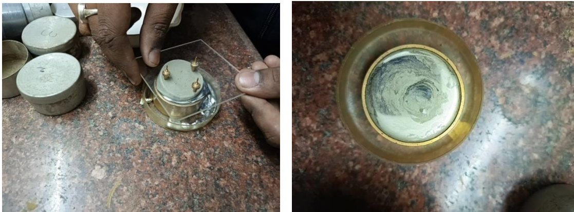
Figure 34 : Shrinkage Limit Test by Mercury Displacement Method
