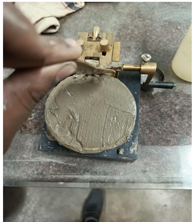
Figure 33 : Plastic Limit Test Using Casagrande Apparatus
