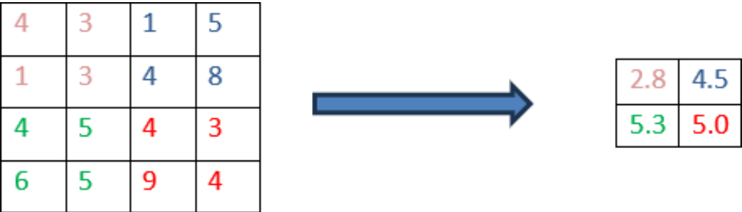
Figure 7: Average Pooling operation Source – Self-prepared using MS word 2016
